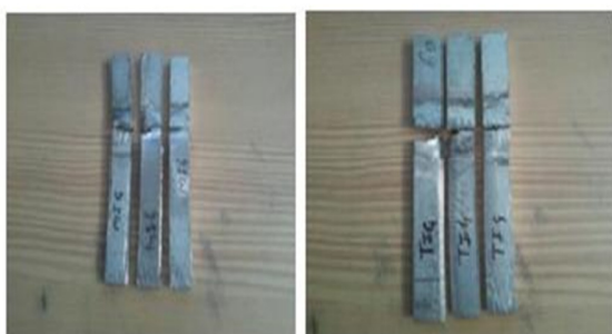
Fig. 6 MIG and TIG weld specimen after Izod test
